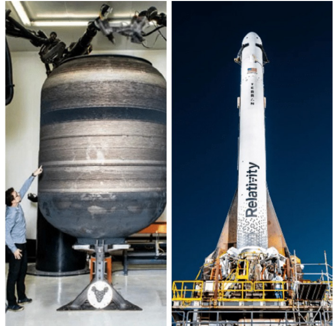
Figure 2. 3D printing technology enables the creation of rocket tanks with unparalleled precision [5] .
