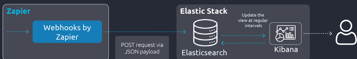
Figure 9: Automated dashboards with Elastic Stack
