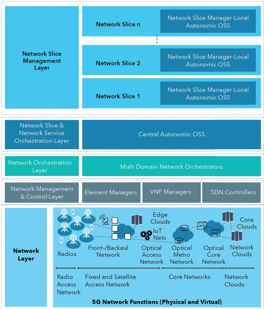
Figure 6: Overall OSS Architecture for 5G
