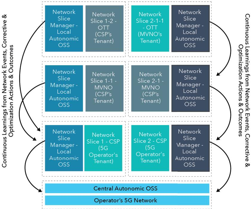
Figure 7: Recursive OSS Systems for 5G Network Operations
