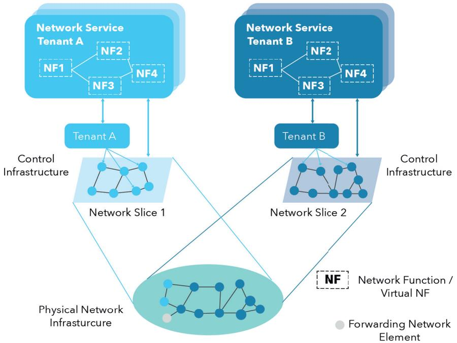
Figure 1: Network Slicing Concept
