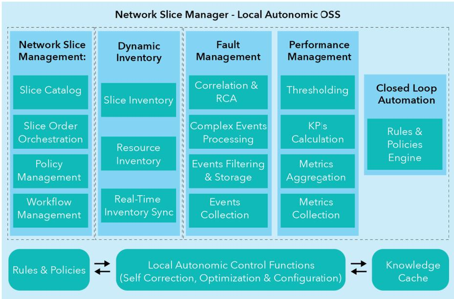
Figure 9: Functional Architecture - Local Autonomous OSS
