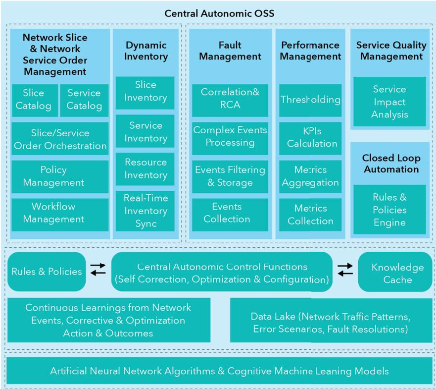
Figure 8: Functional Architecture - Central Autonomic OSS
