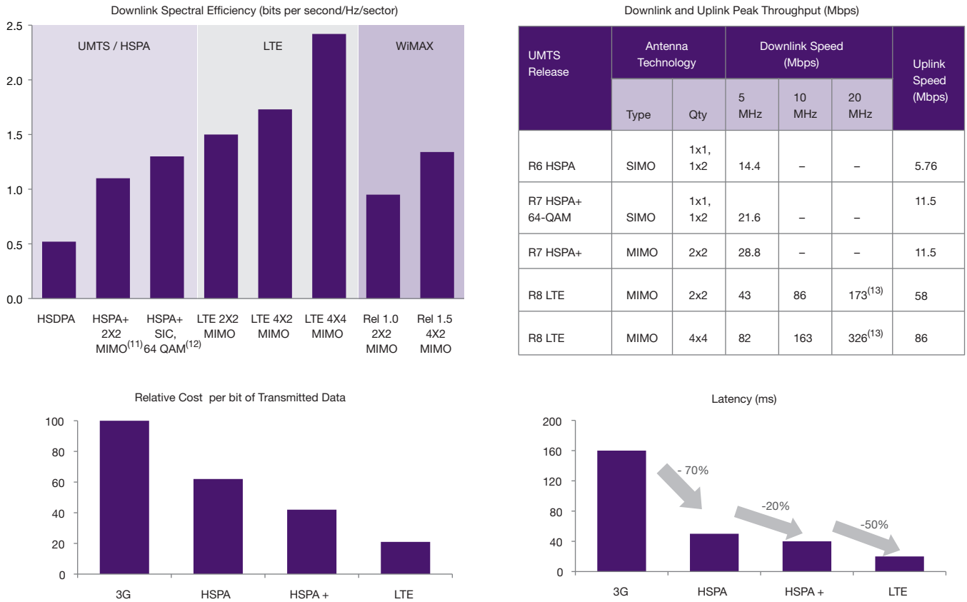
Figure 2: Comparison of LTE Peak Theoretical Throughput, Latency, Spectral Efficiency and Relative Cost per Bit Parameters with Other Mobile Network Technologies
