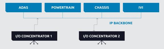
An alternative to this approach is to use the same topology, but to allow features to be distributed across the processors arbitrarily and not necessarily by domain.
