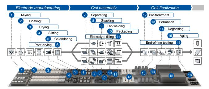
Figure 9: Production process of lithium-ion battery cells
