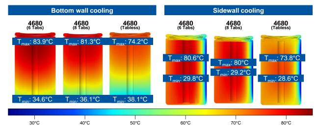
Figure 13: Comparison of bottom and sidewall cooling for steady state results for 3C continuous charging and identical cooling loop efficiency<sup>9</sup>
