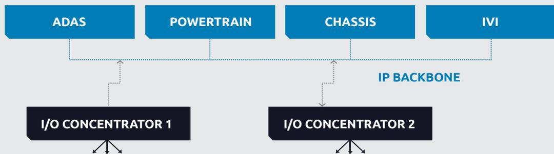
An alternative to this approach is to use the same topology, but to allow features to be distributed across the processors arbitrarily and not necessarily by domain.
