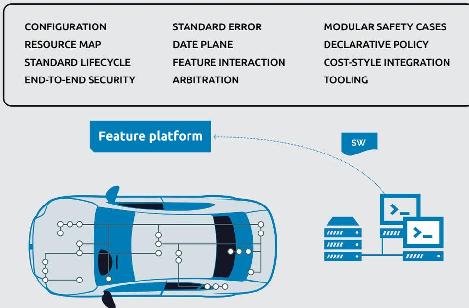
The overall approach is to make the vehicle a software platform as a means to recognize the weight of feature to be delivered by software, and to allow the flexibility of such a software approach to be realized in a controlled, safe, and secure manner.
